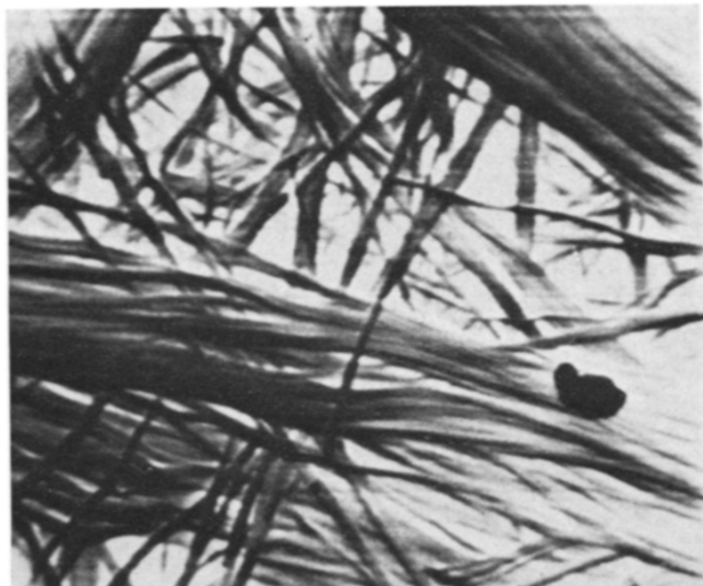
Fig. 7. Electron micrograph of a sample of fibrous cerium(IV) phosphate (magnification 10,000 \times ).
